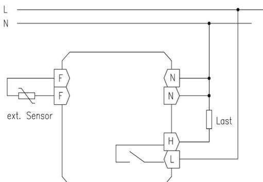
PA-UP Temperature Regulator with numeric scala FRe F2A/50 (Article No. 93088)
