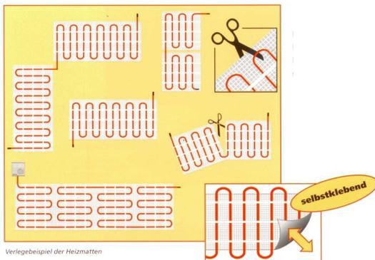
Important! Do not damage the heating cable. Bend the heating map where you cut it and install it in parallel with the first web.
