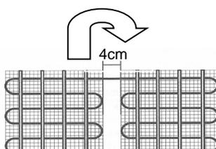
Do not lay heating mats so that they cross each other. Wherever possible, avoid stepping on the heating mats during installation.
